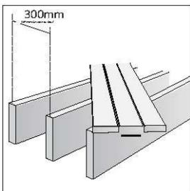
The distance between support rails or joists must not exceed 40cm. (30cm when laying the boards diagonally to the joist). Classic boards must not be used above ground floor applications, unless built on a solid load bearing surface: e.g. a concrete balcony or roof terrace.
