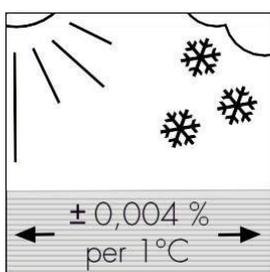
A detailed expansion table can be found on the Technical Data Sheet. However, a rough guide is to leave a 6mm gap at the ends of 4m long boards if installed in mid European spring temperatures (temperature of the boards about 20°C – 30°C).
